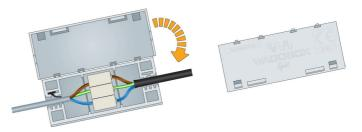
8. If required the WAGOBOX Light can be fitted to a surface using the WAGOBOX mounting button feature. The base of the WAGOBOX Light has two sliding slots, either one or both can be used. Simply fix the mounting button to the
