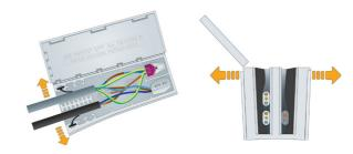
7. Try to keep cables of a similar size together in the same slot and simply push them into the slot as far as they will go.
