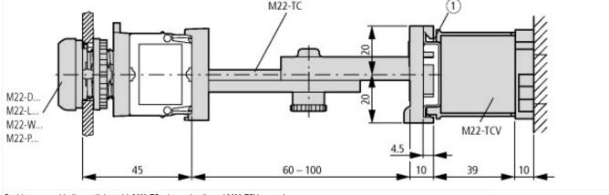
Pushbuttons and indicator lights with M22-TC telescopic clip and M22-TCV extension 1 Top-hat rail to IEC/EN 60715
