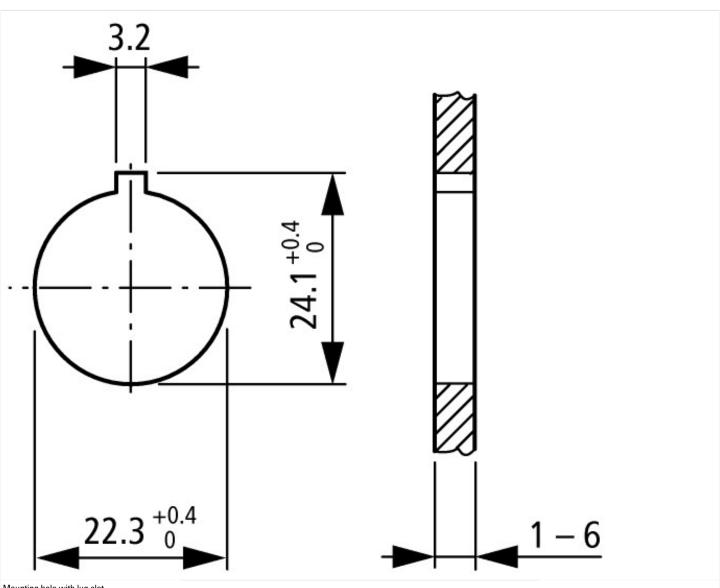
Mounting hole with lug slot
