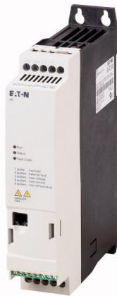
**Variable speed starter, Rated operational voltage 230 V AC, 1-phase, Ie 2.3 A, 0.37 kW, 0.5 HP, Radio interference suppression filter**
