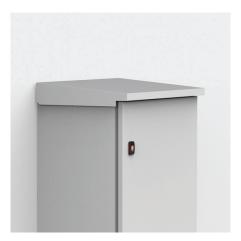
**Description:** To be fitted as an outdoor shelter on single mounted enclosures. The roof is slightly sloped and has a dripstrip. Machining is required. It increases the enclosure dimension in H:60 mm, D:20 mm and W:20 mm.
