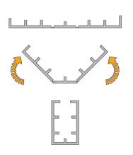
The adapters are supplied flat. To use, fold into a rectangular shape with the side fins facing inward. Insert into the connector receptacle.
