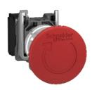
Harmony XB4, Emergency stop switching off, metal, red mushroom Ø40, Ø22, trigger latching turn to release, 1 NC
