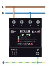
Series connection of ESP 120 D1, ESP 240 D1 and ESP 277 D1 to single phase supplies up to 125 A (fuses not shown for clarity).
