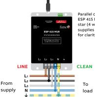
Parallel connection of ESP 415 M1R to three phase star (4 wire and earth) supplies (fuses not shown for clarity).
