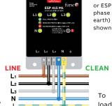
Parallel connection of ESP 415 M1, ESP 208 M1 or ESP 480 M1 to three phase star (4 wire and earth) supplies (fuses not shown for clarity).
