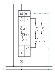
or control voltage 230 V with glow lamp current up to 5 mA
