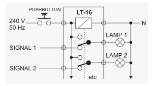
The above diagram shows the operating principle, All signals must be the same voltage and phase
