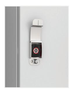
**Description:** The padlocking cover is mounted over the existing standard lock. The standard lock is totally covered and not accessible when padlock is fitted. Maximum padlock bow diameter of 10 mm.
