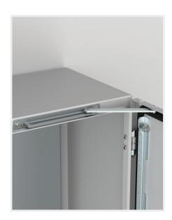
**Description:** Door stop to fit all wall mounted enclosure dimensions. To secure the door in an open position to the degree that meets user requirements. Door stop can be mounted at the top or bottom of the enclosure. Machining is required. Minimum enclosure width  $\geq$  300 mm.
