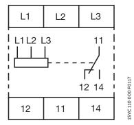
L1, L2, L3Control supply voltage = measuring voltage11-12/14Output contacts - closed-circuit principle
